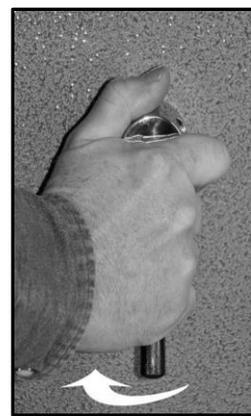
2. Install the temporary spoke handle. (Note: handle not needed on single lever safes)
