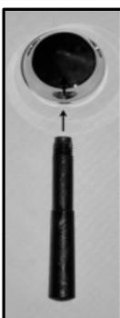
5. Remove the temporary handle & add a drop of Handle Thread Lock to the ends of metal spokes and install.
